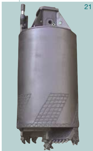
Rock type drilling bucket with calibration collar type BEES-K 1060
