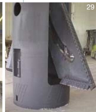
Cutting arm with flat teeth
