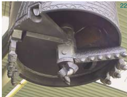
Swivelled bottom gate of an EMDE drilling bucket
